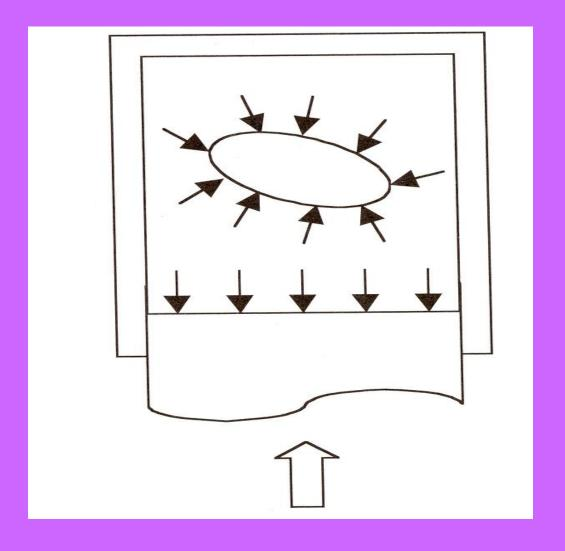
The isostatic principle in high pressure processing
