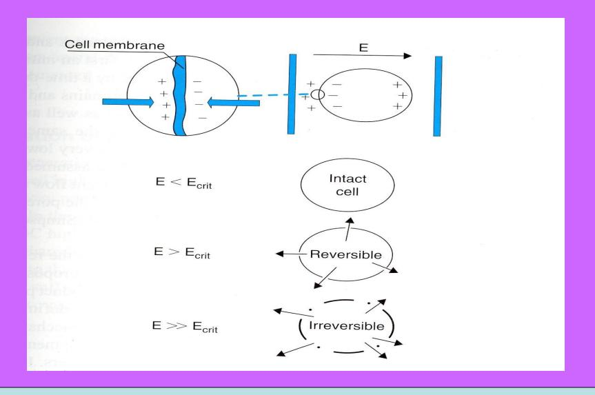
Schematic depiction of mechanism of membrane permeabilization by electrocompressive forces induced by an external electrical field. Increasing treatment intensity will lead to formation of large, irreversible membrane pores
