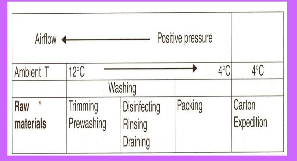
Temperature gradient and air flow in the processing unit
